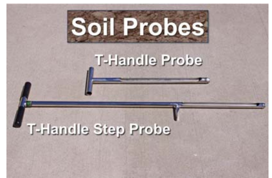
Figure 4: Soil probes provide a simple method for collecting soil samples. Photo by Joe Boggs.
