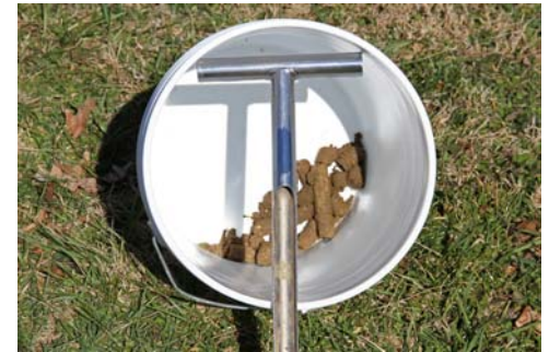
Figure 7: Soil samples should be collected in a clean plastic bucket. Photo by Joe Boggs.
