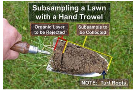
Figure 6: Using a hand trowel for soil sampling. Photo by Joe Boggs.
